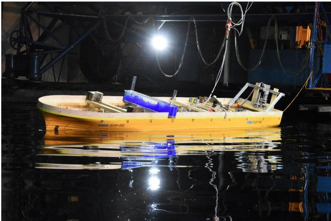
Figure 4: HSVA HERM model test of a 9,000-TEU container vessel equipped with a Hoppe FLUME tank design
