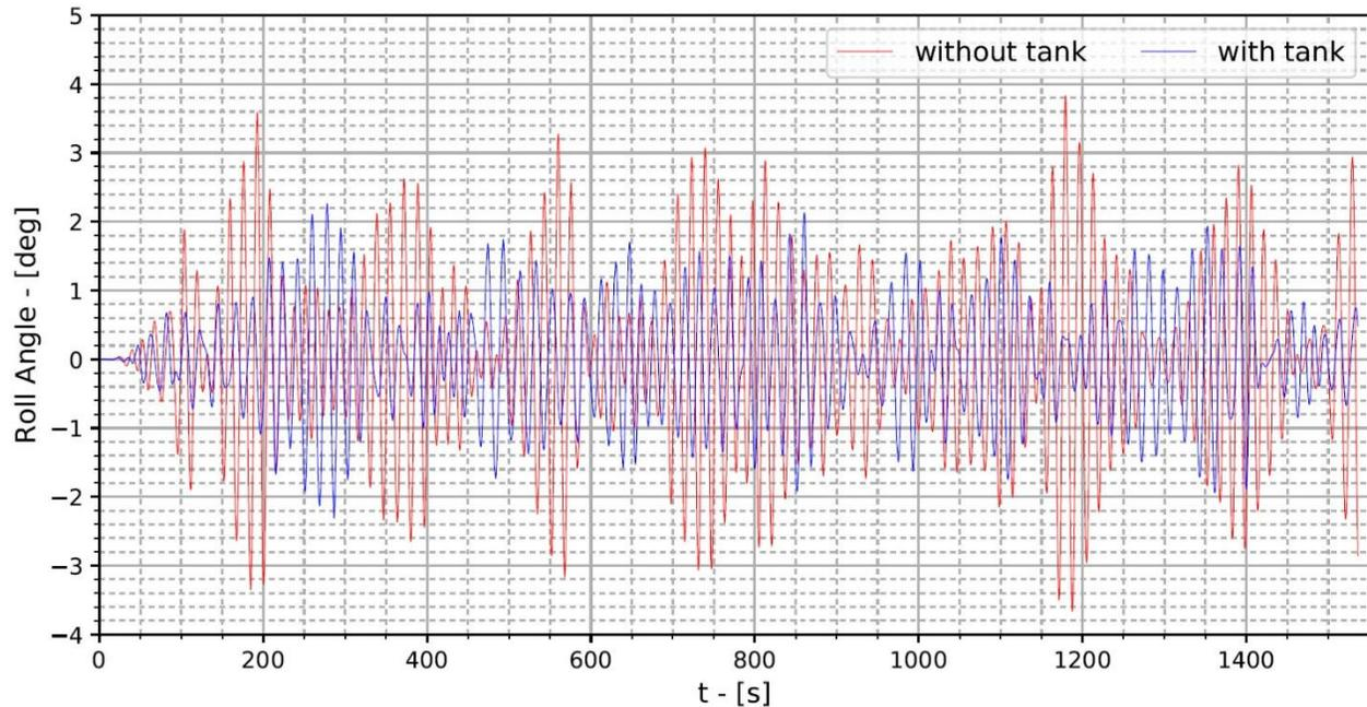
Figure 2: Time domain analysis showing the influence of a FLUME tank on the roll motion of a 9,000 TEU container vessel
