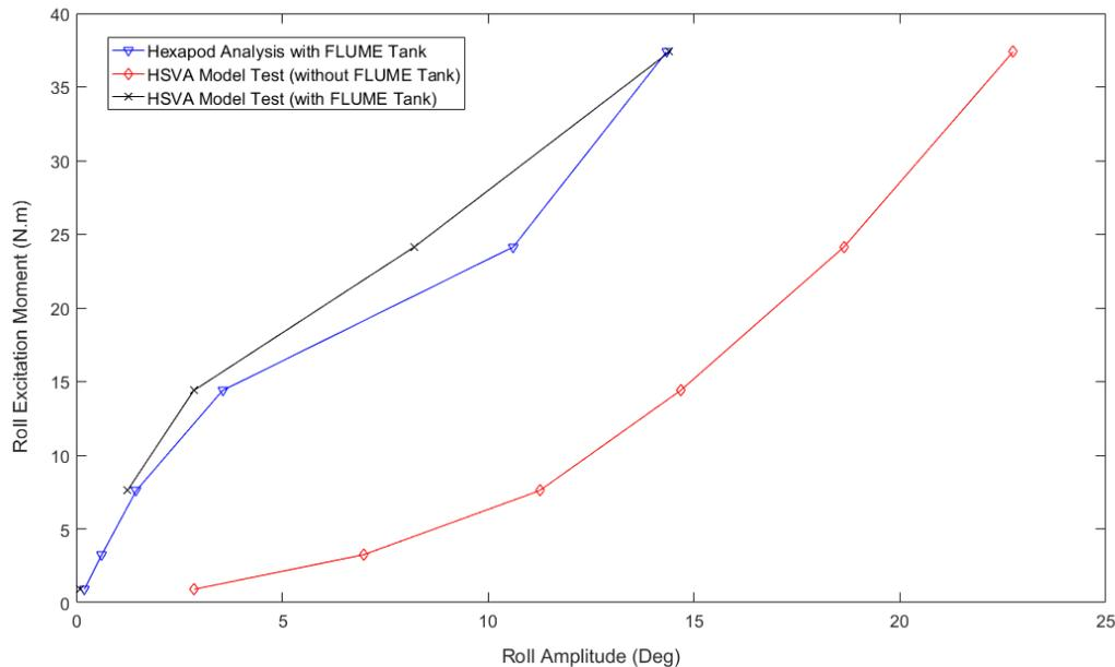
Figure 3: Comparison between experiment using a FLUME tank directly with the ship model and the method in which the FLUME tank Hexapod test results are added numerically to vessel motions without a tank
