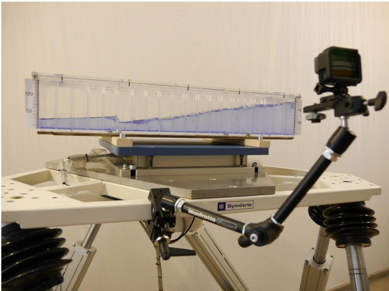
Figure 1: FLUME roll damping tank for a 9,000 TEU container vessel design mounted on the hexapod
